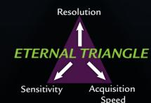
A new approach is Airyscanning, which images the diffraction-limited illumination point (Airy disk) with an area detector, rather than a single-point detector. In Airyscanning, emission light is not blocked by a pinhole, thereby enhancing sensitivity, speed, and resolution.
